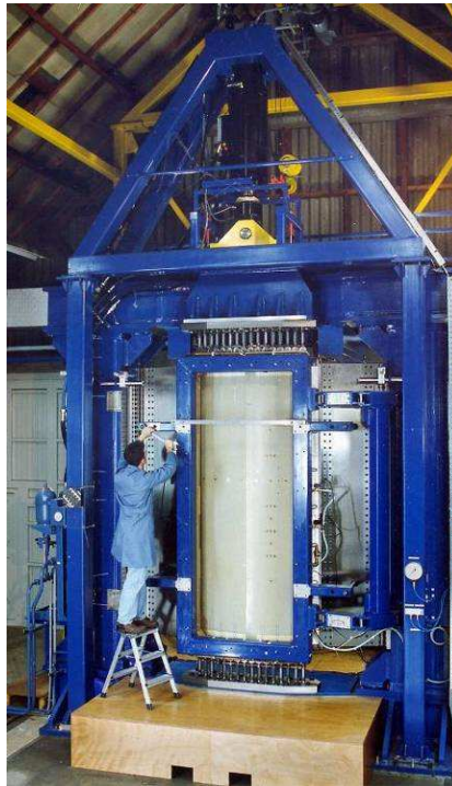
Test set-up for the testing of fuselage panels
