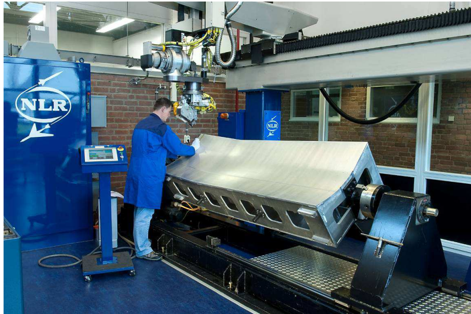
Advanced Fibre Placement machine with jig for the manufacturing of a composite wing panel
