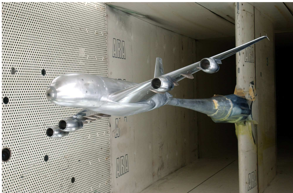
Airbus A380 Model in the ARA Transonic Wind Tunnel
