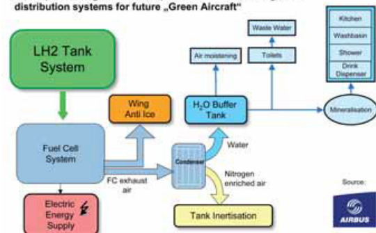
Conceptual design and development of the LH2 storage and distribution systems for future „Green Aircraft“
