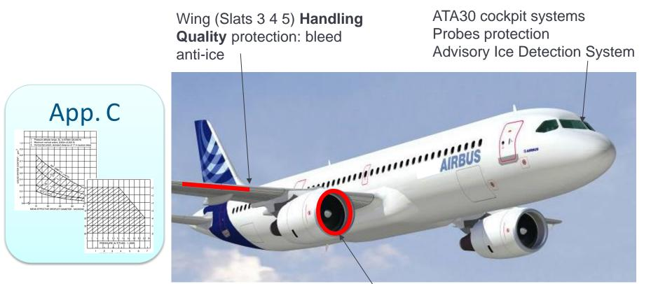
Nacelle inlet cowl Foreign Object Damage protection: bleed anti-ice
